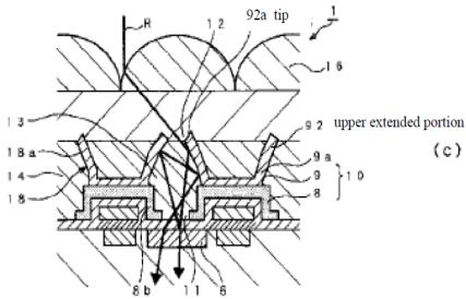
J.A. 461. Sony's petition further explained that element 9 is a "second light shielding film," having "lateral faces 9a" that are approximately vertical surfaces, and upper extended portions 92. J.A. 122–123 (citing Abe ¶¶ 38, 47). Sony provided the following annotation of Figure 3 to support its contention that this figure discloses a trapezoidal reflecting wall:
